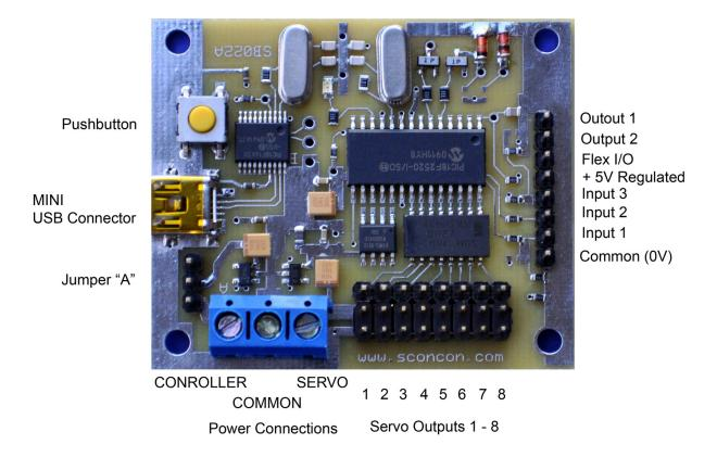
Note: SB022S version shown; SB022M includes servo outputs only.
